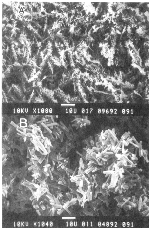
Figure 4. SEM micrographs of (A) poly(ester-amide) 6a prepared in Marlotherm-S at 350 °C/16 h and (B) poly(ester-amide) 6d .
